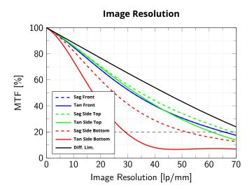
Modulation Transfer Function (MTF) vs. Image Resolution, wavelength range 486 nm - 656 nm of cylindrical object of diameter 30 mm and height of 20 mm
